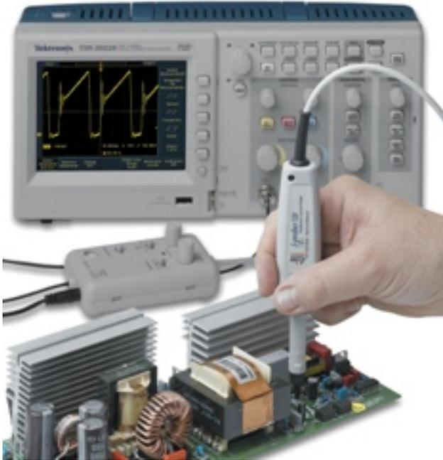
Saelig has announced the Aim-TTi I-Prober 520, a unique, compact hand-held current probe for use with any oscilloscope, unlike any other current measurement device available. The current flowing in a pcb track can be observed and measured, allowing measurements by merely placing the insulated tip of the probe on to the track.
