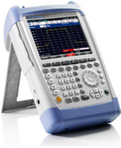
The R&S FSH4 and R&S FSH8 handheld analyzers from Rohde & Schwarz offer comprehensive new functions for detailed measurements in LTE networks. With these handheld spectrum analyzers, users can now perform modulation analysis in the LTE frequency division duplex (FDD) and time division duplex (TDD) modes.
