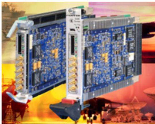
Pentek, Inc. today unveiled the first in a family of ruggedized boards for high-performance military and avionics applications utilizing the industry's most advanced FPGA technology. Pentek's 53xxx Cobalt™ board family incorporates Xilinx's Virtex-6 FPGAs for on-board signal processing, delivering digital sampling rates to 1 GHz in a compact 3U VPX form factor.
