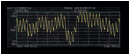
Figure 7. A phase-modulated plot of the “settled” PLL frequency. The 20-degree phase shifts can contribute to bit errors in quadrature-modulated devices.
