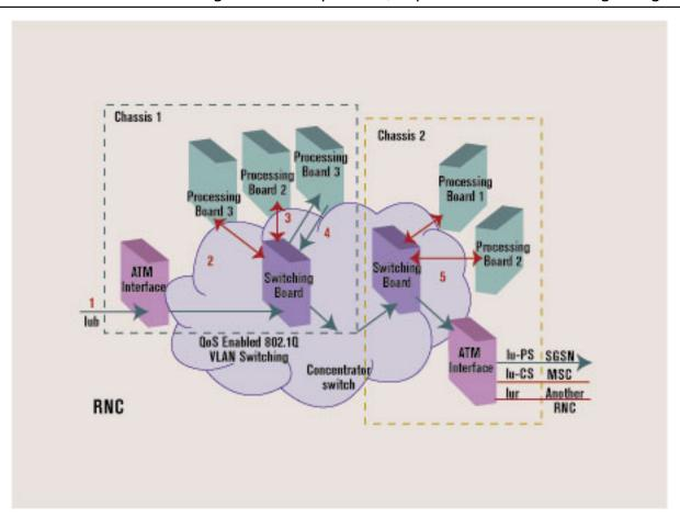
Figure 1. Architecture of RNC and its QoS Solution.
