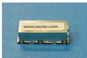
Integrated Microwave introduces a ceramic diplexer (Model Number 930073) operating in the 2.4 GHz band. Channel BW is 10 MHz, and loss is 2.5 dBa. The 10 dB BW is 75 MHz. TX/RX isolation is 22 dB. This miniature diplexer offers 2 poles per channel, handles 5 W CW and measures 1.1&#215 0.470&#215 0.310. SMT package is standard. Options include custom frequencies and rejection points.
