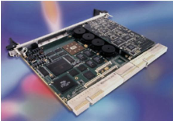
Ixthos, Inc., has announced a new line of digital radio boards for telecoms-intensive applications. The new highly integrated, software programmable CHAMP-DR/T<sup>®</sup> boards provide four channel receivers or dual channel transceivers (transmitters/receivers), tightly coupled to up to four PowerPC G4 with AltiVec), or four TI high end C6x digital signal processors (DSPs) in a single 6U VME or CompactPCI slot.
