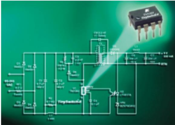
Power Integrations, Inc announced the availability of a new generation of energy efficient, low power off-line switcher ICs. The new family of devices, named TinySwitch-II, maintains the simplicity of the previous TinySwitch line while providing additional features and lowering system cost. The output power capability has also been increased to 23 Watts (15 Watts with a universal input), making it an ideal energy efficient, cost-effective solution addressing most standby power requirements.
