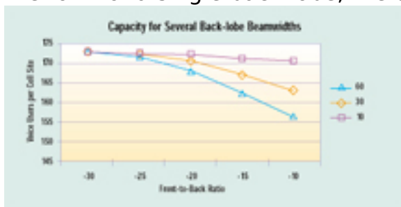
Figure 6. Capacity predictions for a typical three sector cell site configuration rotated by 30 degrees. The different lines are for the back-lobe beamwidths 60, 30 and 10 degrees.
