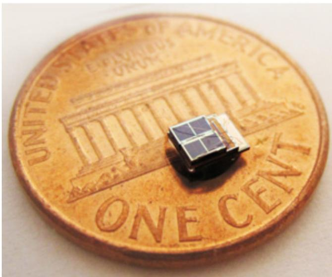
*Figure 1. This smart sensor system measures just 9 mm<sup>3</sup>*
