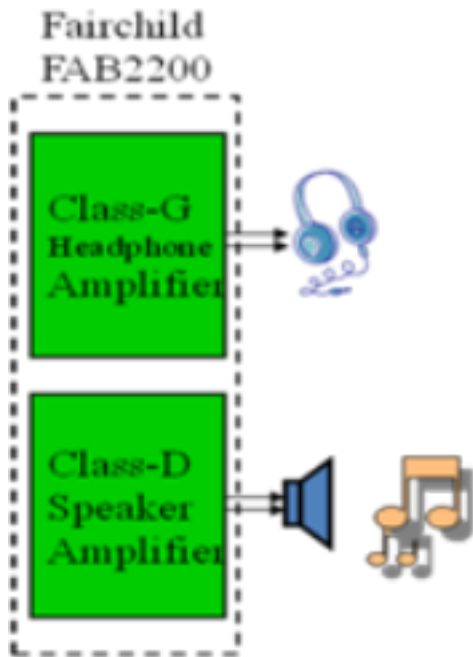
Figure 12. Audio sub-system ICs merge speaker and headphone amps on same die
